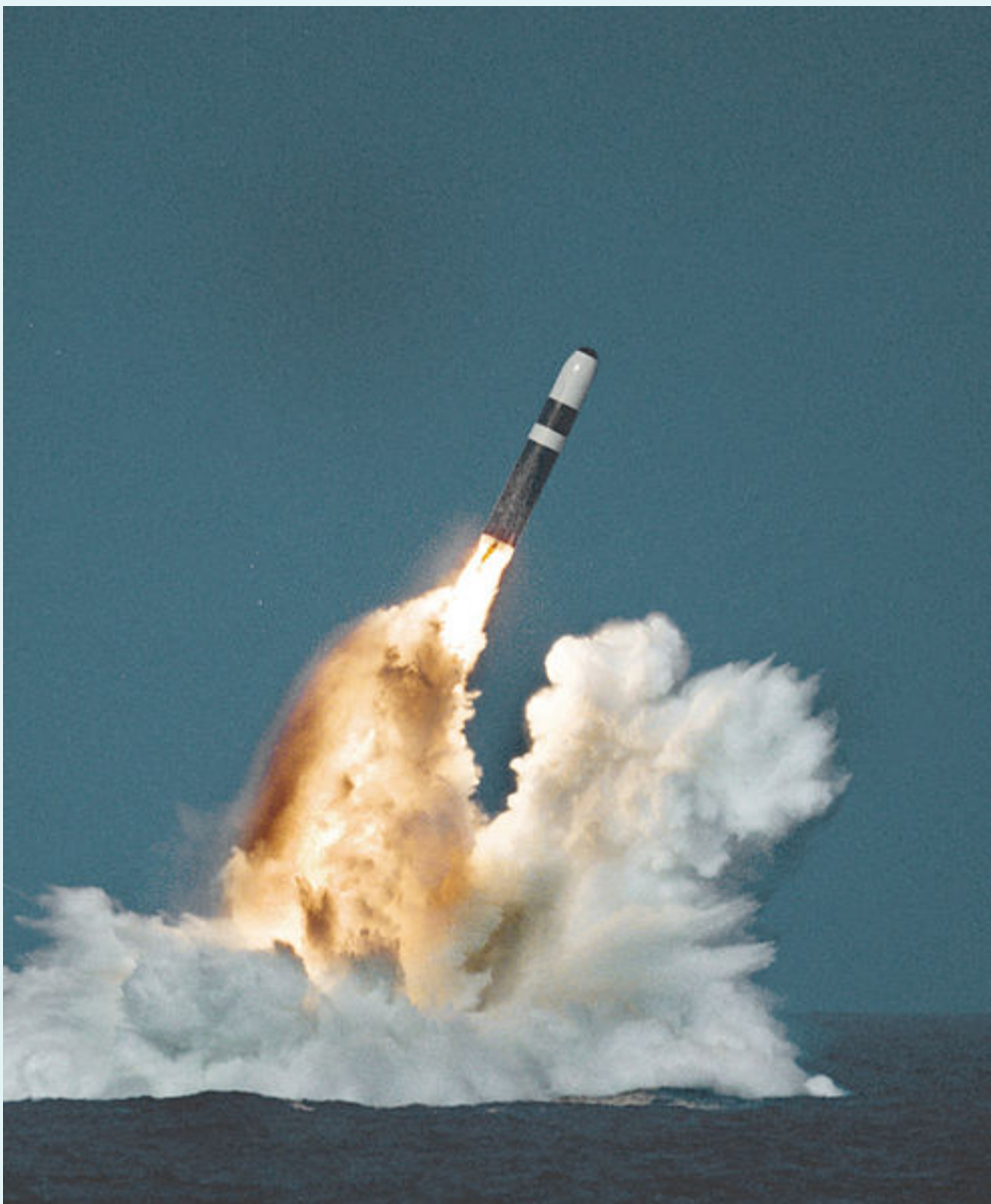
A Trident II missile fires its first stage SRB after an underwater launch from a Royal Navy
