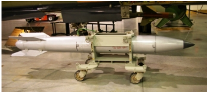
B61 training unit accurately replicates the shape and size of a "live" B61 | Credit: Wikimedia Commons
