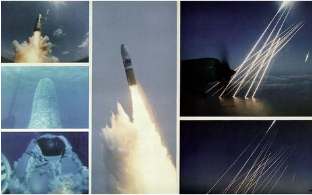
Montage of an inert test of a United States Trident SLBM (submarine launched ballistic missile), from submerged to the terminal, or re-entry phase, of the multiple independently targetable reentry vehicles. Photo Credit: Wikimedia Commons
